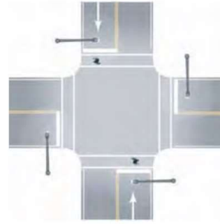
B. Alternative layout – Better for visibility of pedestrians, but harder to illuminate conflict areas in the intersection.
