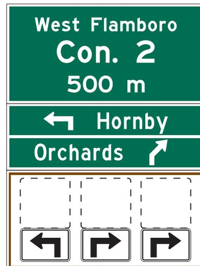
(d) **Turn-Off Guide and Information Sign Assembly with Roadway Identification and Services Marker Board**
