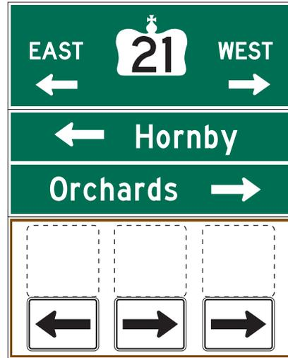
**(a) Advance Guide and Information Sign Assembly with Roadway Identification, Destination and Services Marker Board**
