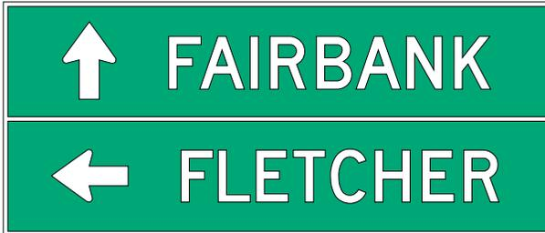
Since the sign is 30 m from the turning point, the speed reduction can continue for 30 m after the sign is passed. Therefore, required legibility distance can be reduced by 30 m to 113 m.
